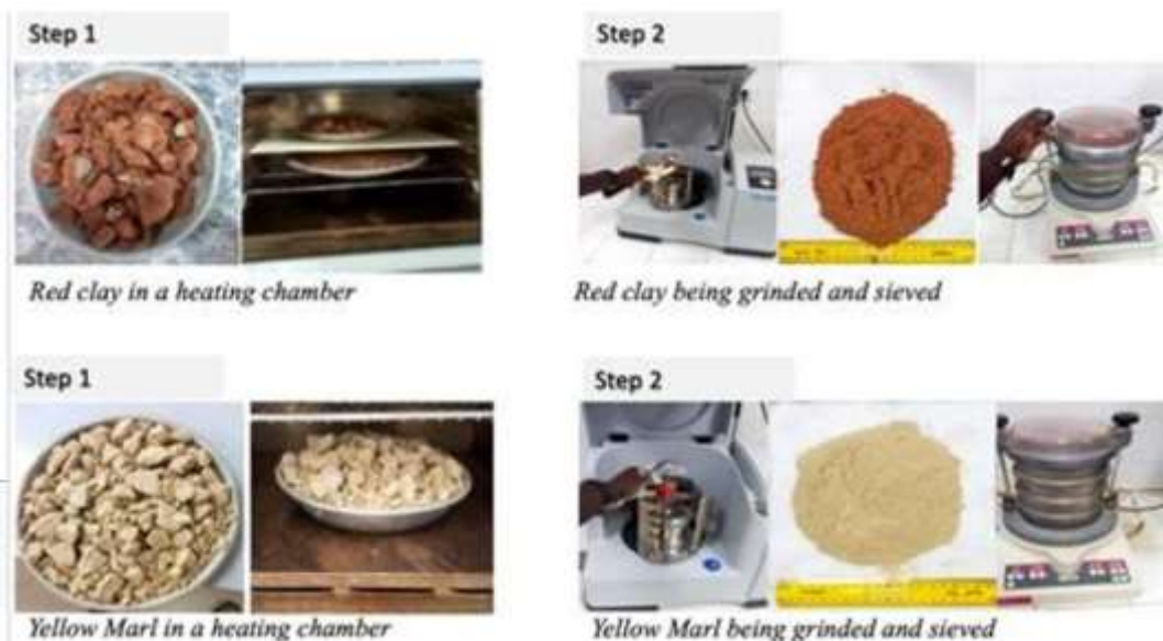
Figure 4. Steps 1 and 2 of the brick fabrication process.
