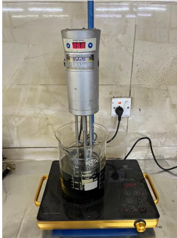
Figure 2. Wet process modification of modified asphalt with crumb rubber.
