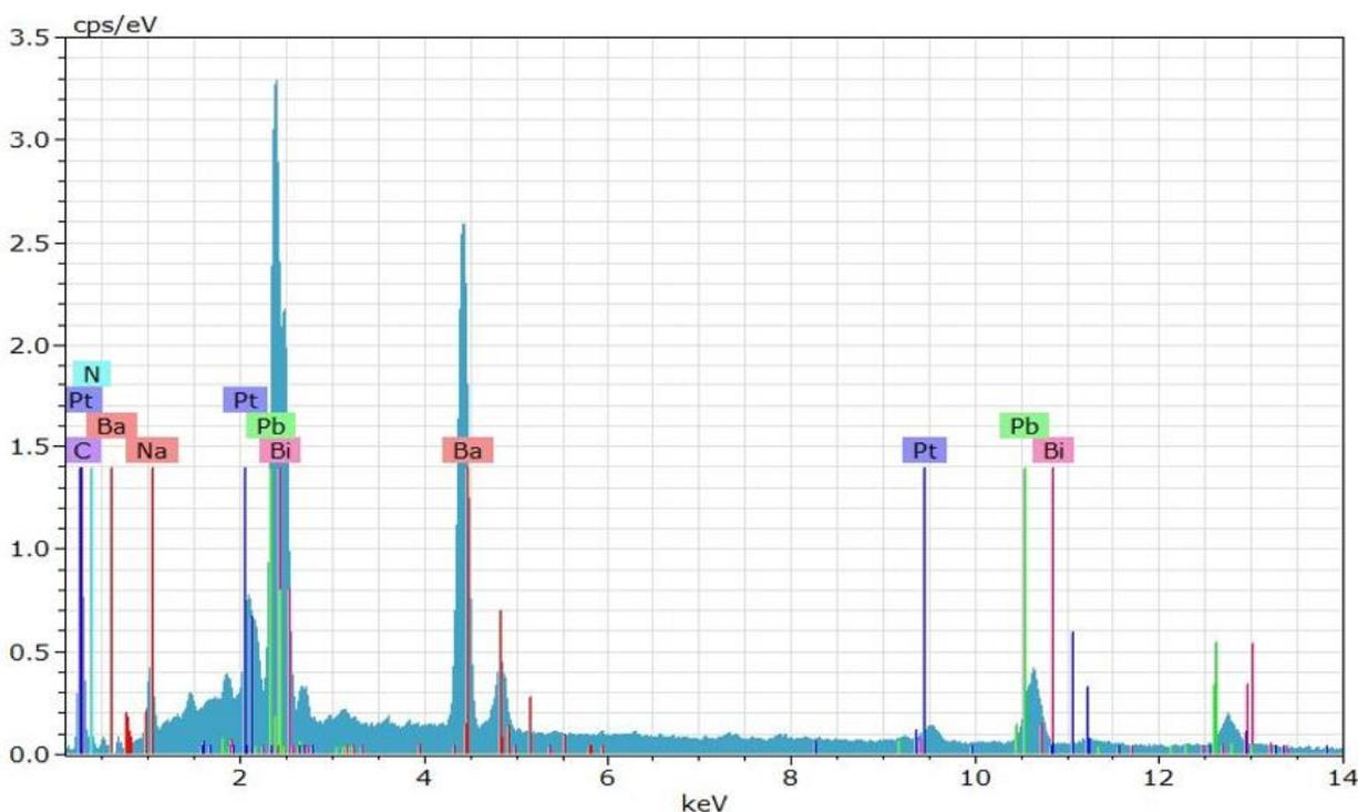
**Figure 6.** Show the EDX surface micrograph of point one of new ferroelectric compound.
