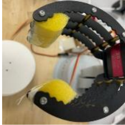
Figure 6. Gripper modified with soft sponge padding.
