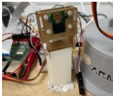
Figure 7. Gripper modified with soft sponge padding.
