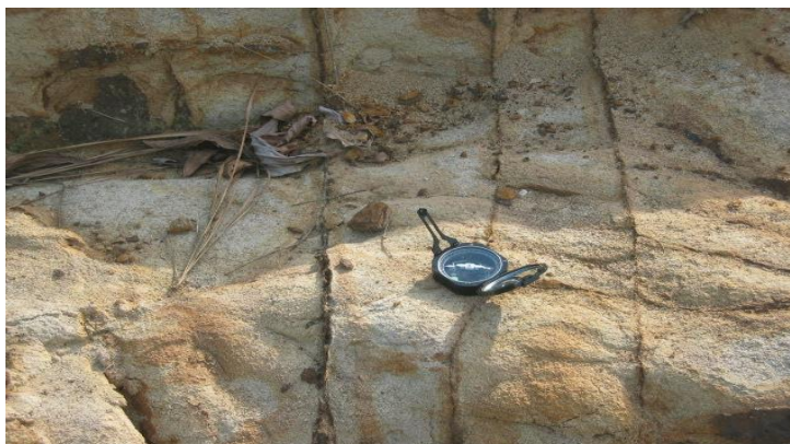
Figure 3. Brittle sandstone with spacing between 10 centimeters to 80 centimeters.
