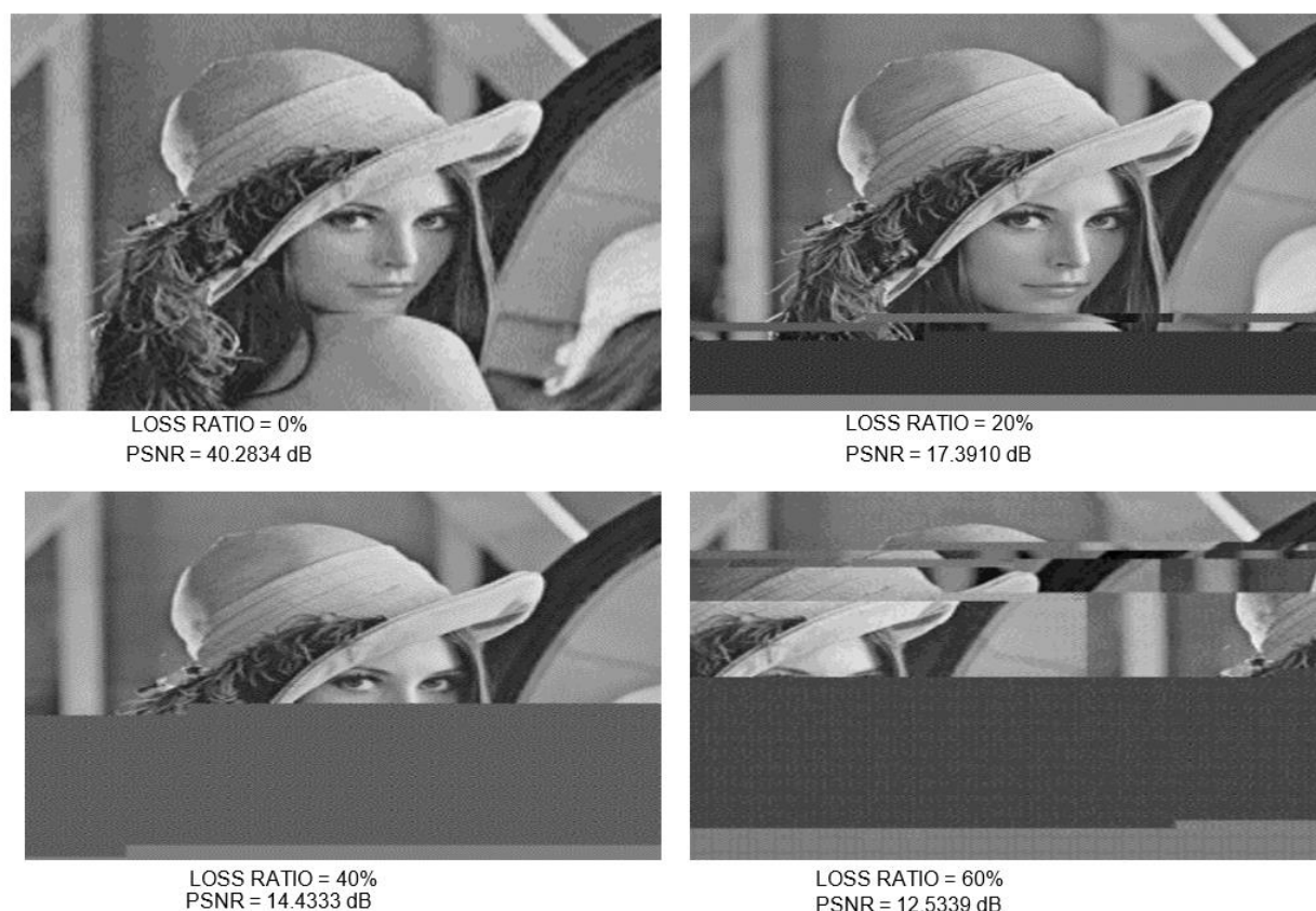
Figure 11. The quality of received images at various packet loss ratios.
