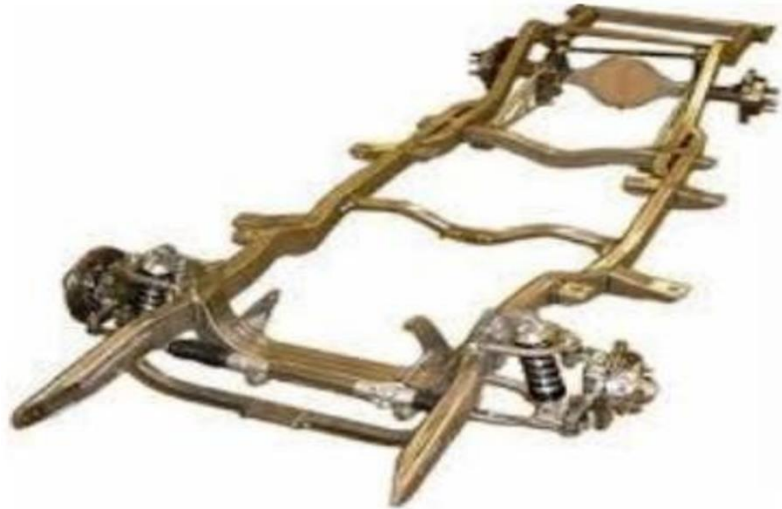
Figure 1. Schematic of the ladder-frame chassis.
