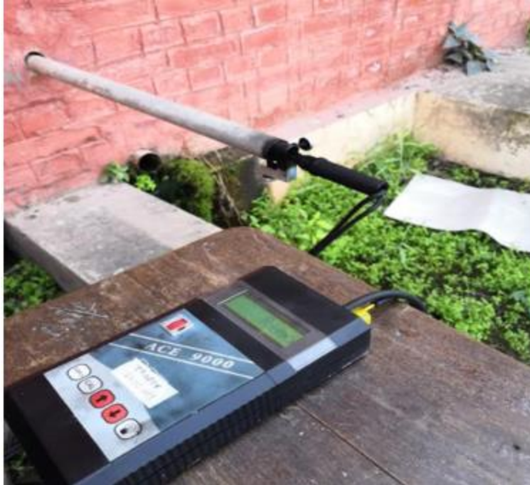
Figure 1. (b): AVL Di-gas Emission analyzer.
