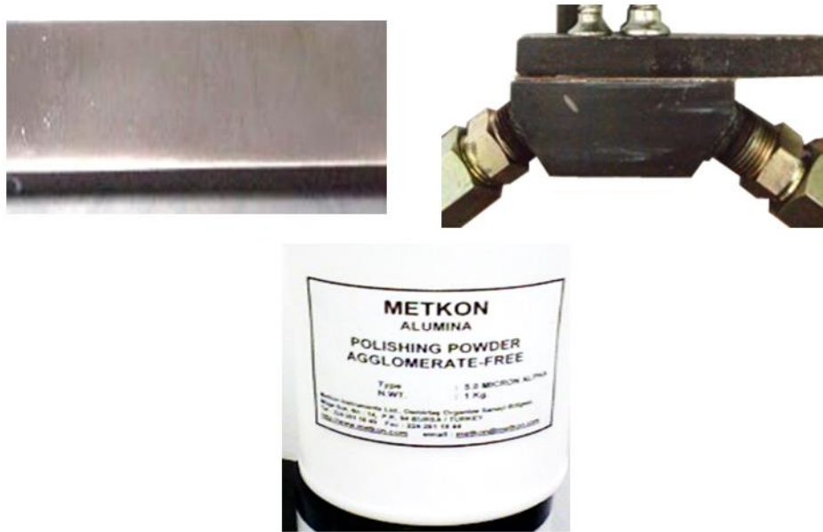
Figure 3. The workpiece, AFM nozzle, and abrasive media ( \text{Al}_2\text{O}_3 +Silicon Oil).
