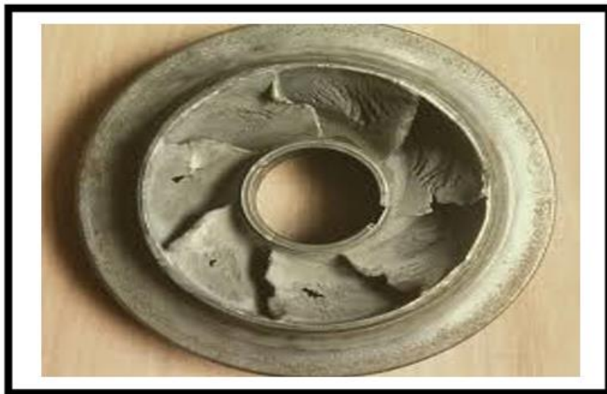
Figure 3. Condition of the wheel very degraded [9].
