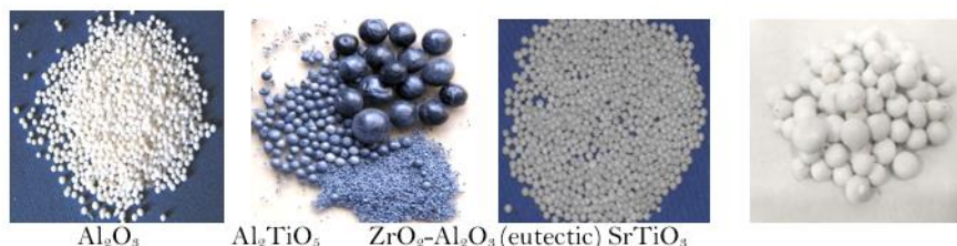
Figure 2. Materials, obtained by melting and hardening in the LSF (Parkent) according to the scheme with the slope angle of the water-cooled substrate \approx 30^\circ .
