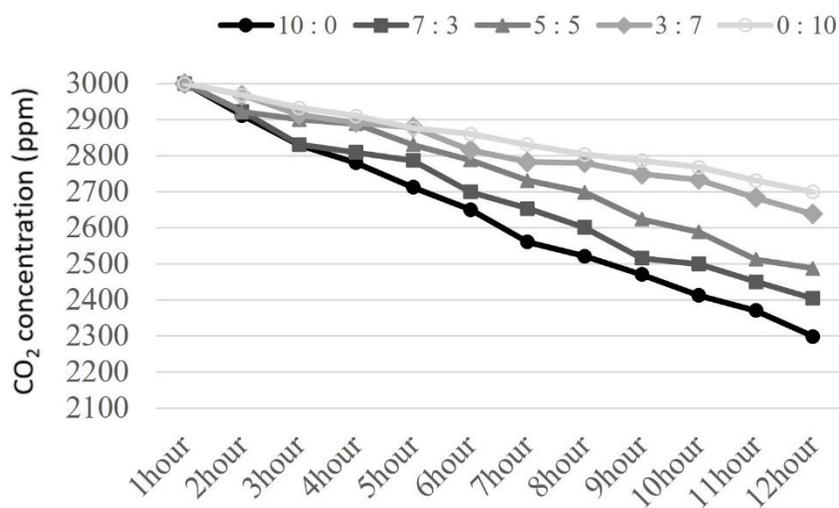
**Figure 5.** CO<sub>2</sub> reduction ratio of cement composite substituted MEA according to BFS and FA ratio.
