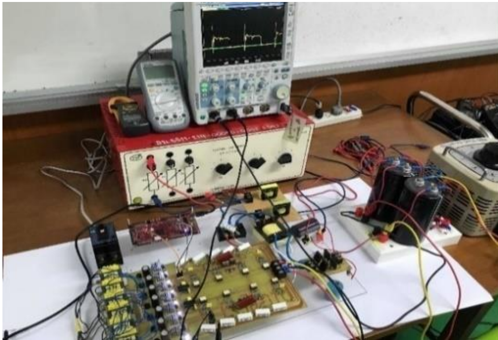
Figure 5. Experiments on boost converter and snubber.
