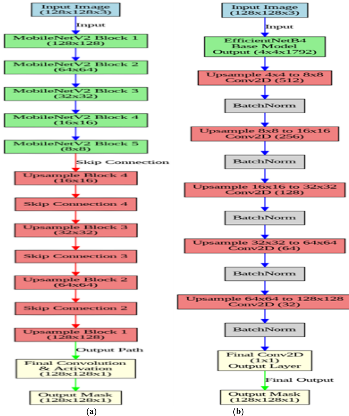
Figure 2. (a) U-Net with MobileNetV2 Encoder and Pix2Pix Decoder (b) Simple DeepLabV3+ Architecture Using EfficientNetB4.
