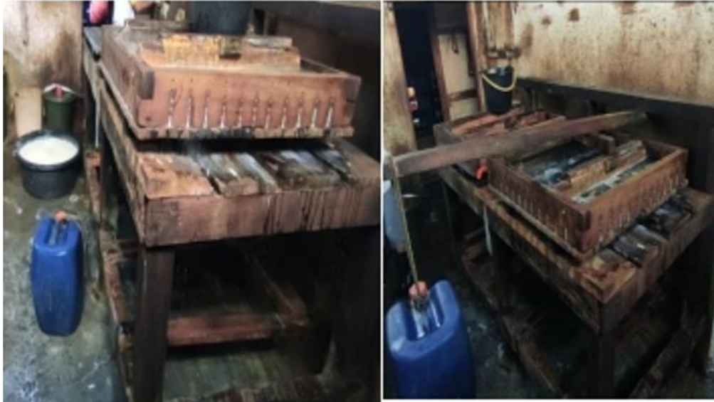
Figure 6. Position of Sari Tahu container under mold (Left), manual press tool (Right).
