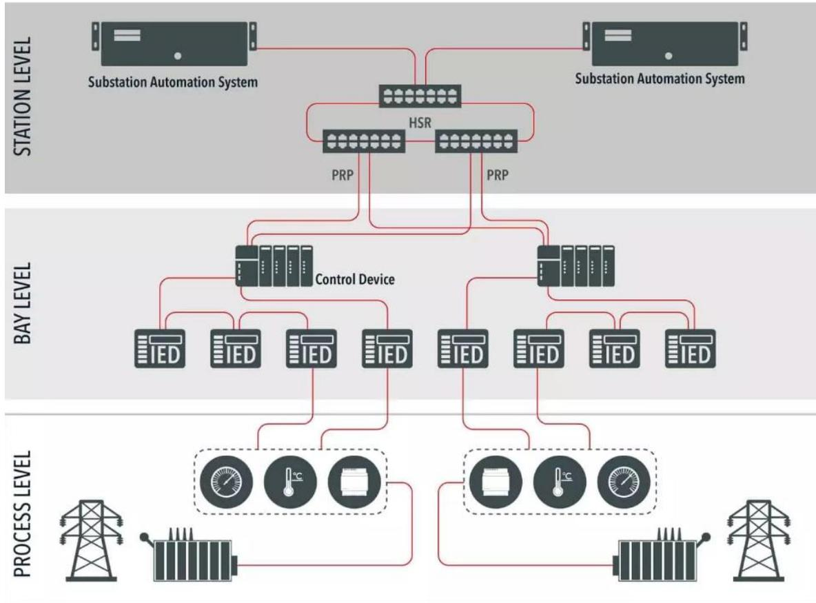
**Figure 3.** Substation architecture configuration for IEDs with 61850 standards.
