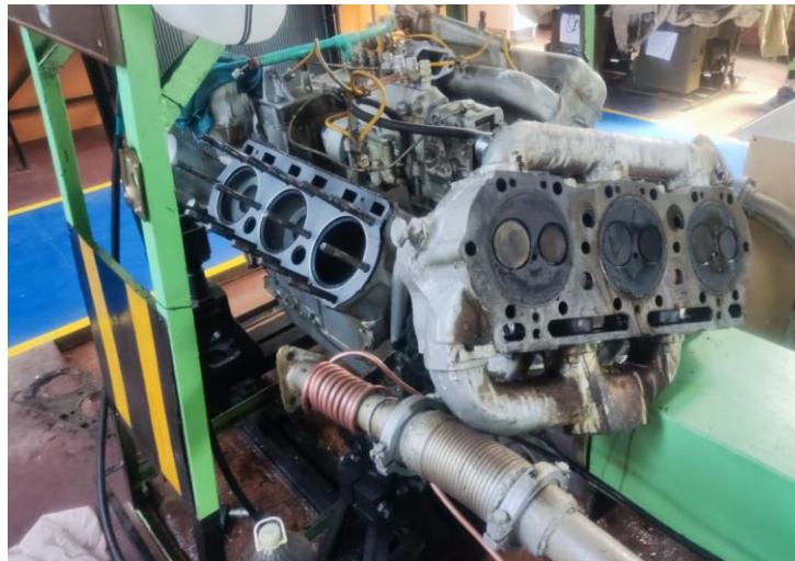
Figure 10. External view of the process of partial disassembly of the DEU (YaMZ-236D-3).
