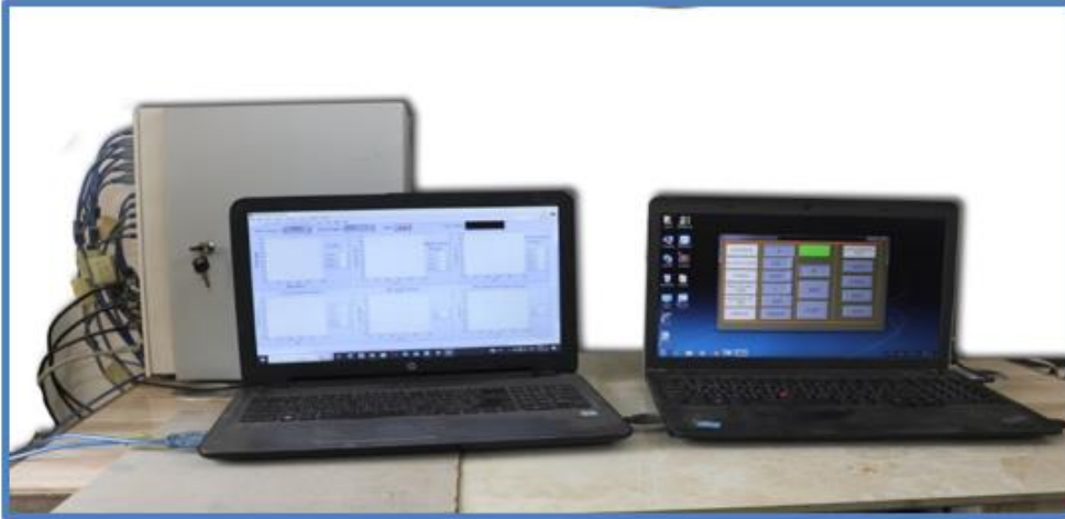
(a) Computer-controlled data logger
