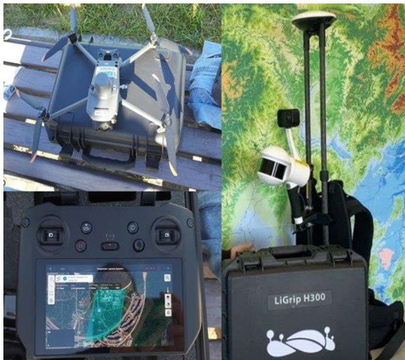
Figure 2. Devices which were used in the work (on the right - UAV, on the left - laser SLAM-scanner with backpack).
