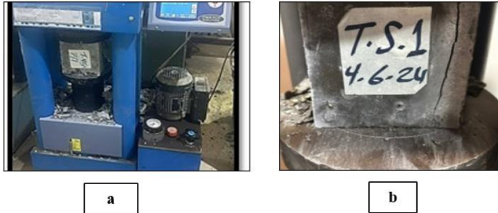
Figure 6. Compression Strength Test: (a) Compression Apparatus (b) Tested Specimen.
