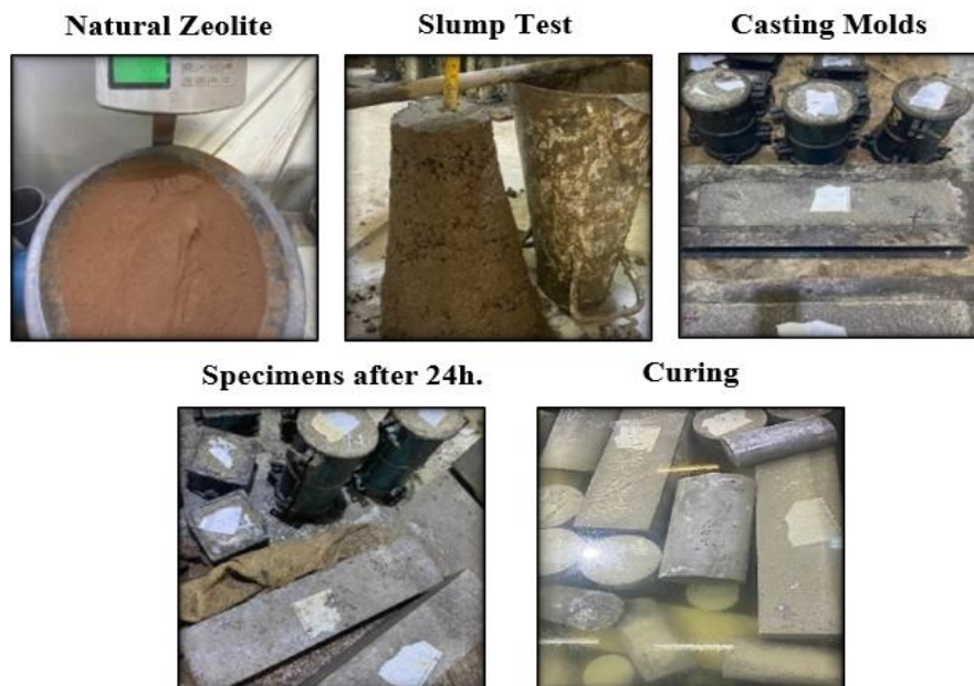
Figure 4. Special concrete mix with natural zeolite process.
