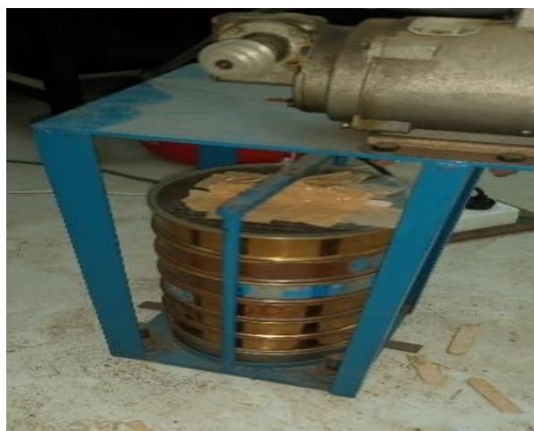
Figure 2. Sieve shaker with stack of sieves from sieve No.4 to No. 200.
