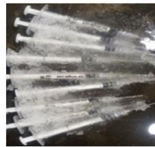
2) COVID-19 syringes after being immersed in liquid nitrogen.
