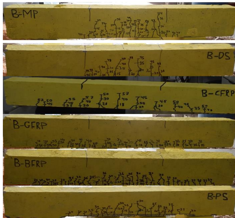
Figure 7. Cracking pattern for beam samples.
