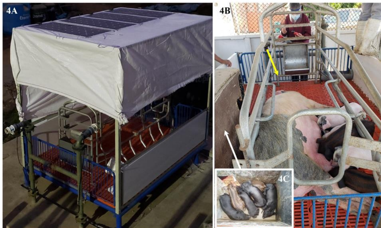
Figure 4. Functional breastfeeding module with geothermal system energy. (4A) UNJFSC Breastfeeding Module. (4B) Sow in comfort. The yellow arrow shows the exit of the cooled air from the geothermal coil. (4C) Piglets sleeping in comfort on a functional resistance plate with photovoltaic energy. The white arrow indicates the piglets' nest.
