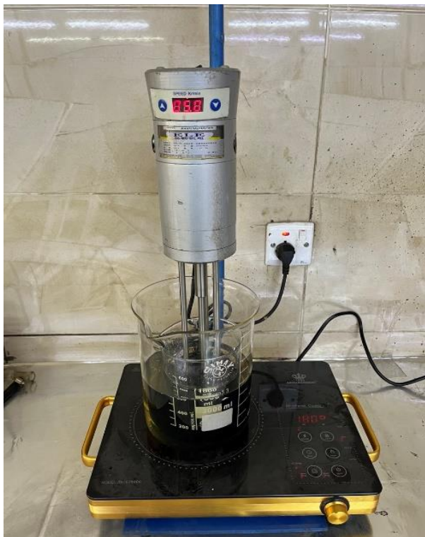
Figure 1. Wet process modification of modified Asphalt with Sasobit
