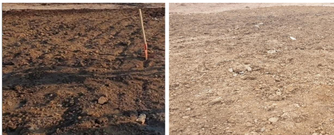
Figure 5. Plot with contaminated soil before bioremediation (left) and after application of the biopreparation after 12 weeks (right).
