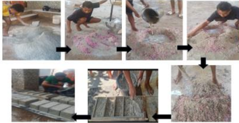
Figure 5. Process of mixing materials to molding bricks.
