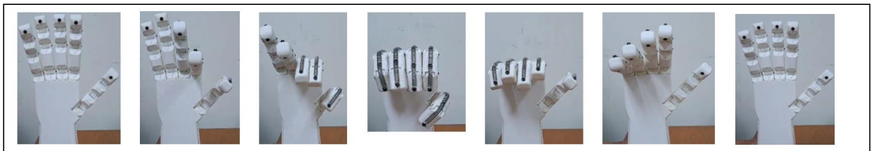
Figure 5. All the fingers Open from Thumb and close from Thumb.
