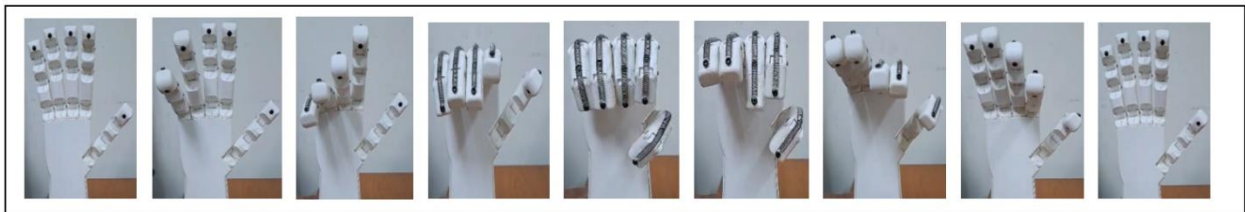
Figure 4. All the fingers Open from Pinky finger and close from Pinky finger.
