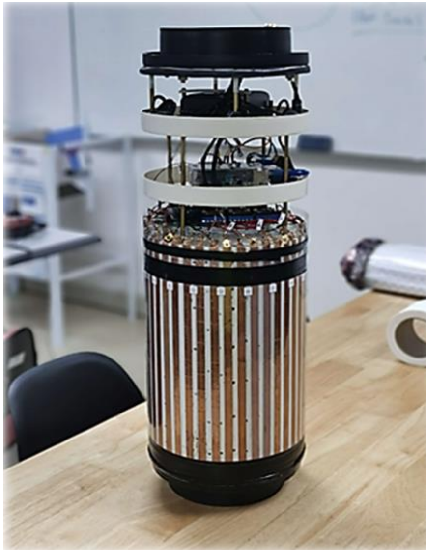
Figure 2. Actual USV prototype with capacitive plates around the circumference.
