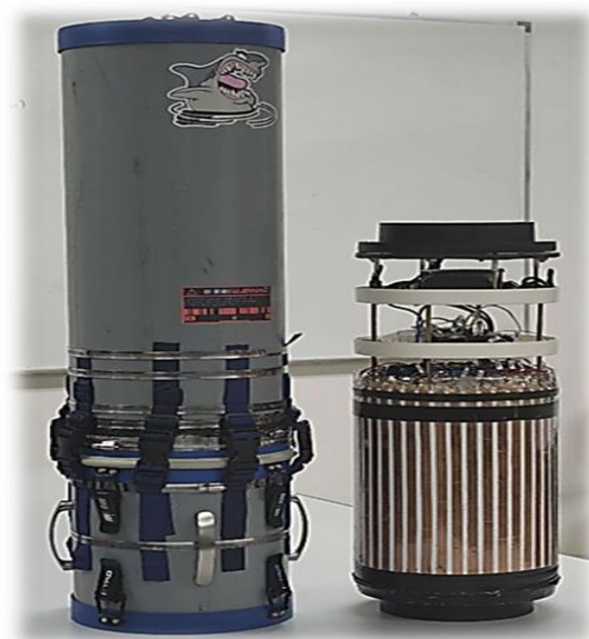
Figure 3. USV external UPVC casing to enclose the capacitive sensors.
