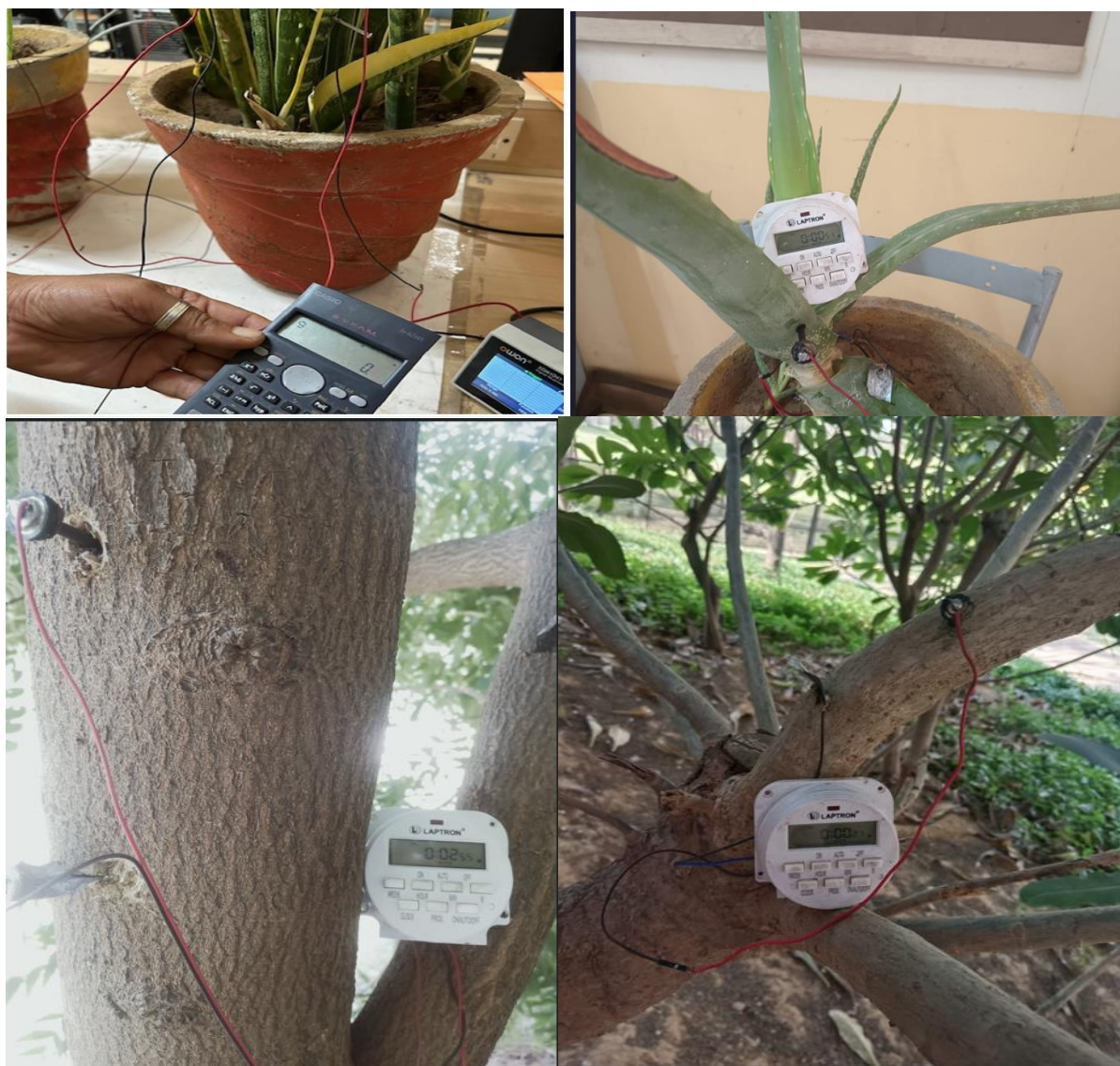
Figure 4. (c): Application of harvested potential from plant/trees to power up sensor
